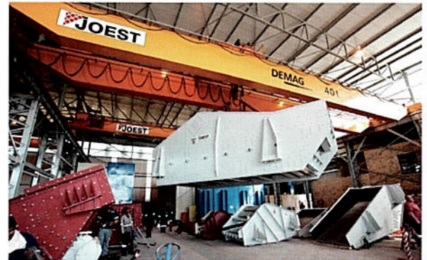
A typical large-width banana screen in Joest's Kempton Park, Johannesburg facility that is destined for a colliery in South Africa.
