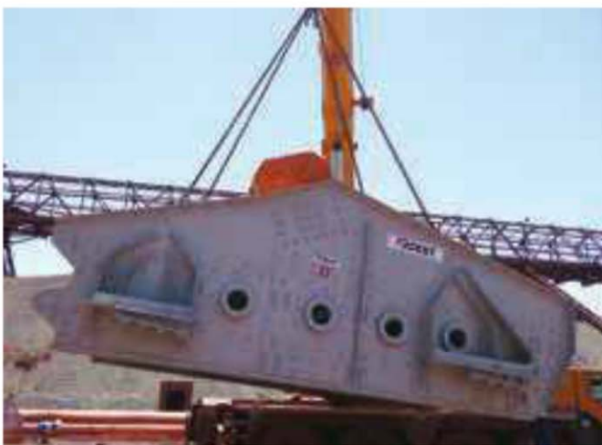
A dense media recovery screen from Joest being delivered for an iron ore application.
