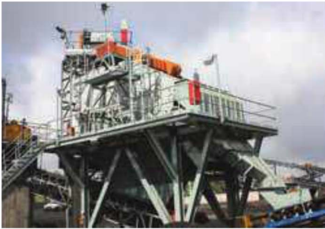
A Joest double deck-vibrating screen of up to 4.3 m for a coal application.
