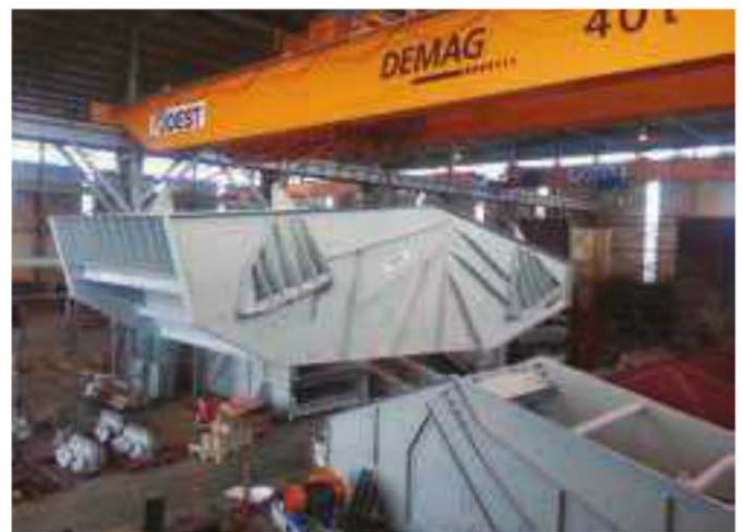
A banana screen for a gold application in Liberia under construction at Joest’s Spartan premises.
