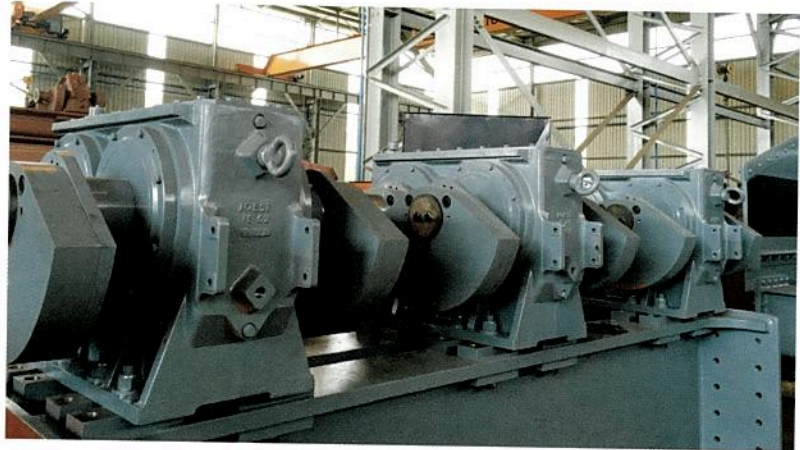
Joest's large exciter gearboxes that will drive the massive scalping screen.
