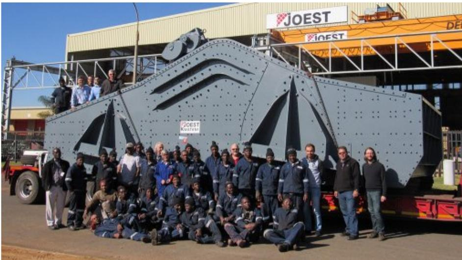
Company Announcement - Large tonnage throughputs, long drop heights, very heavy R.O.M. ore boulders and large cut sizes all mean that the screen and its component parts must be specifically designed for the loads and stresses normally not experienced in dry screening processes. Kenny Mayhew-Ridgers, general
