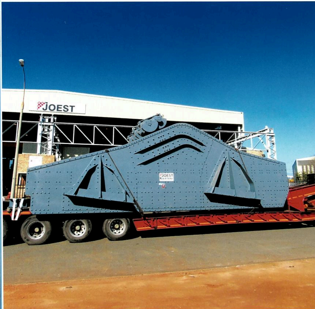
This large scalping screen will handle variable ore conditions with a continuous feed load of 6 000 tph
