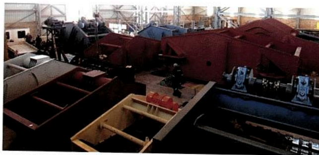
The Joest Kwatani screens were customised to match the exacting metallurgical requirements of the client's processes and the associated mechanical duty
