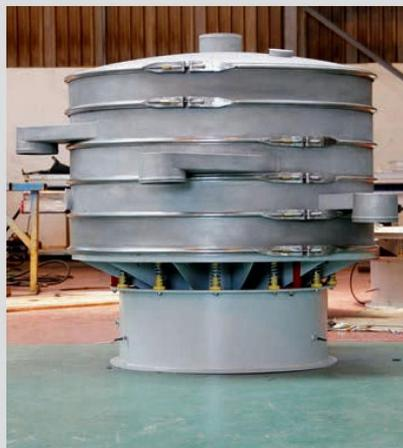
**SWECO round separators have been a mainstay for mining and minerals processing industries and are available from Joest**
