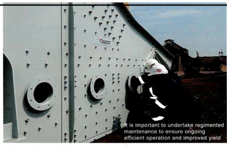
undertake a full audit covering the operating performance and the condition of the screen. "We also consider the upstream processes to ensure that the feed is within the original specifications for which the screen was engineered," says Theresa.
