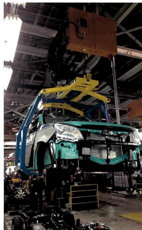
The assembly process saw automotive bodies and chassis from two separate production lines being joined on a single moving line.
