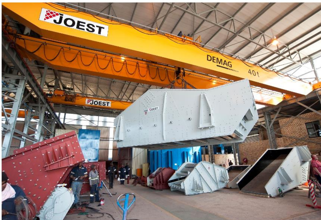
A large-width banana screen in Joest's Kempton Park facility that is destined for a colliery in South Africa
